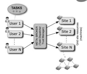
Fig. 1. Model of a security-aware grid system.
