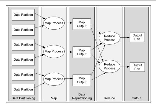
Fig. 1. Computing stages of the MapReduce model.
