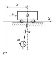
Fig. 1. Planar model of a crane, where M, m, l, u and  $\alpha$  are respectively the masses of a crane and payload, the rope length, the controlling signal corresponding to the control force acting on the crane, and the sway angle of the payload.
