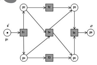
Fig. 3. Workflow net that is sound.
