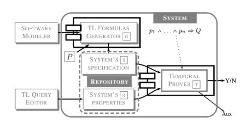
Fig. 2. Architecture of a deduction-based verification system.
