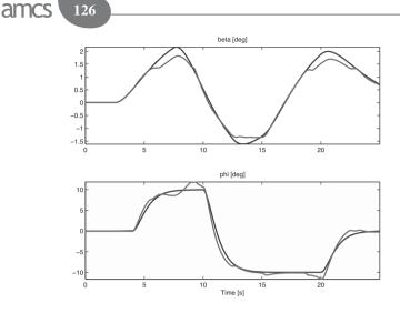
Fig. 11. Output tracking in the complete rudder jamming case using input allocation and fault-dependent scheduling. Black: reference signals filtered by  $hq_{\beta}$ ,  $hq_{\phi}$ , grey: outputs of the GTM model.
