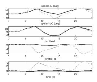
Fig. 14. Comparison of quasi-static allocation vs. dynamic allocation: spoiler and throttle control inputs in the complete rudder jamming case using input allocation and fault-dependent scheduling. Black: baseline reference deflections, grey dashed: real actuator deflections, black dotted: quasi-static allocation deflection demands, light grey dash-dotted: quasi-static real actuator deflections.
