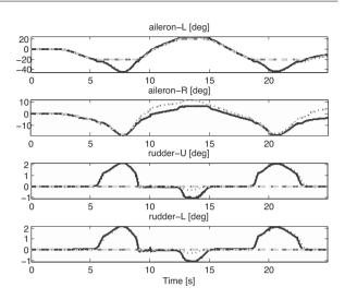
Fig. 13. Comparison of quasi-static allocation vs. dynamic allocation: aileron and rudder control inputs in the complete rudder jamming case using input allocation and fault-dependent scheduling. Black: baseline reference deflections, grey dashed: real actuator deflections, black dotted: quasi-static allocation deflection demands, light grey dash-dotted: quasi-static real actuator deflections.
