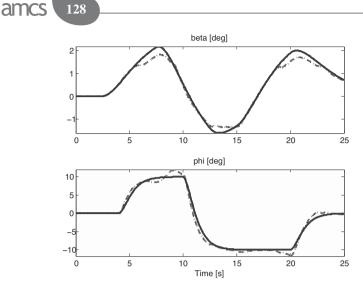
Fig. 18. Comparison of the nominal vs. uncertain system model: output tracking in the complete rudder jamming case using input allocation and fault-dependent scheduling. Black: reference signals filtered by  $hq_{\beta}$ ,  $hq_{\phi}$ , grey dashed: outputs of the GTM model with baseline dynamic allocation, black dotted: outputs of the GTM model with five knots uncertainty in LPV controller scheduling.
