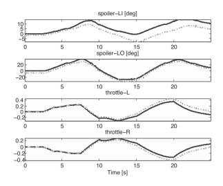
Fig. 17. Comparison of baseline with the FDI offset error case: spoiler and throttle control inputs in complete rudder jamming case using input allocation and faultdependent scheduling. Black: baseline reference deflections, grey dashed: real actuator deflections, black dotted: FDI offset allocation deflection demands, light grey dash-dotted: FDI offset real actuator deflections.
