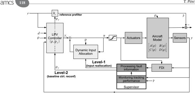
Fig. 1. General architecture of multi-level reconfigurable control.
