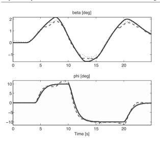
Fig. 15. Comparison of baseline with the FDI offset error case: output tracking in the complete rudder jamming case using input allocation and fault-dependent scheduling. Black: reference signals filtered by  $hq_{\beta}$ ,  $hq_{\phi}$ , grey dashed: outputs of the GTM model with baseline dynamic allocation, black dotted: outputs of the GTM model with FDI offset.
