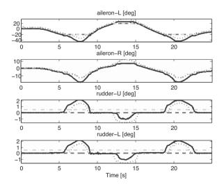
Fig. 16. Comparison of baseline with the FDI offset error case: aileron and rudder control inputs in the complete rudder jamming case using input allocation and faultdependent scheduling. Black: baseline reference deflections, grey dashed: real actuator deflections, black dotted: FDI offset allocation deflection demands, light grey dash-dotted: FDI offset real actuator deflections.
