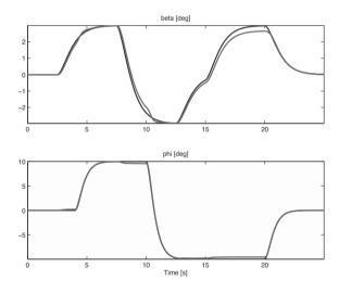
Fig. 5. Output tracking in the upper rudder jamming fault case, input allocation with a baseline controller. Black: reference signals filtered by  $hq_\beta$ ,  $hq_\phi$ , grey: outputs of the GTM model.
