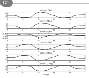
Fig. 4. First six control inputs in the upper rudder jamming fault case, input allocation with a baseline controller. Black: the output of the controller, grey: the saturated input signals. (The negative inputs on the left inboard (LI) and left outboard (LO) spoilers are implemented by deflecting in the positive direction the corresponding right inboard (RI) and right outboard (RO) spoilers.)
