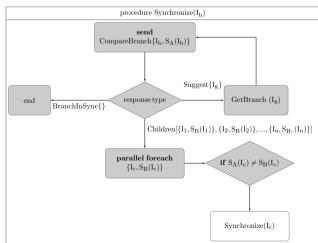
Fig. 5. Simplified synchronization process.
