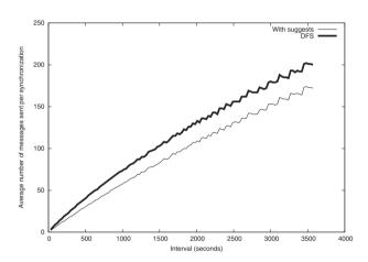
Fig. 11. Performance improvement obtained using the Suggest messages.
