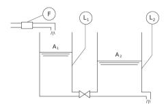
Fig. 1. Two-tank system. F: input flow to tank 1,  $L_1$ ,  $L_2$ : water levels in tank  $A_1$ ,  $A_2$ : surface areas in tanks 1 and 2.
