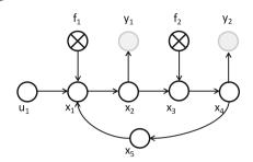
Fig. 2. Example GP graph. x: process variables,  $u_1$ : input, y: outputs,  $s_1(y_1, u_1)$ ,  $s_2(y_2, u_1)$ : diagnostic signals  $(es_{1,2}(f_1) = \langle s_1, s_2 \rangle, es_{1,2}(f_2) = \langle s_2, s_1 \rangle)$ .
