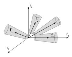
Fig. 3. Direction characteristic for faults in the residual space.
