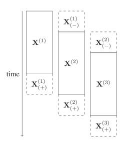
Fig. 1. Schematic representation of a data flow in the sliding window mechanism. In the picture the time flows from top to bottom. Subsequent windows are placed from left to right. Each multivariate data sample forms a row of a matrix.
