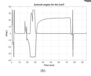
Fig. 10. Control signals from the control allocation method: forces (a), azimuth angles (b).
